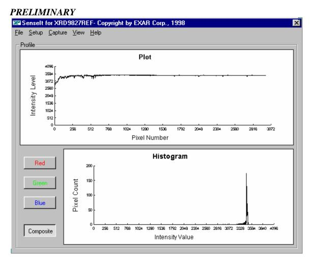
Figure 10. White Target Scan Without Gain Adjustment
